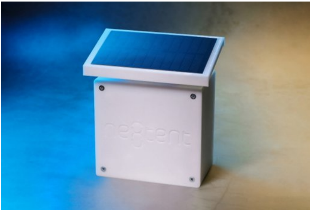
Figure 3.6 - Nextent eKo Bluetooth/WiFi Sensor (Image Courtesy of Inocess)
