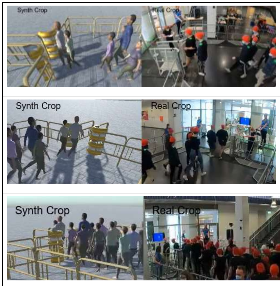
Figure 1. Real crowds captured within this project in a laboratory setting (right) are tracked to obtain 2D trajectories of each individual. We then convert 2D tracks into 3D articulated humans (left), which is used as training data for data-driven methods to analyze dense crowds.
