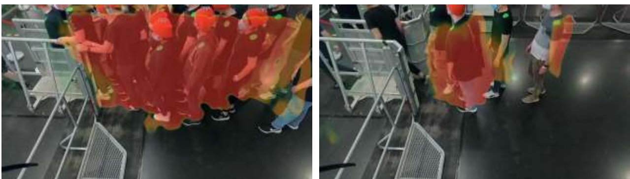
Figure 6. Qualitative results on real-world data. Our model outputs a colormap per-frame that highlights the parts of the image where persons are not moving at the normal velocity. Here, people waiting to go through the bottleneck scenario are detected.
