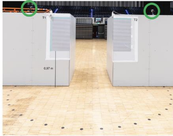
Figure 2. Front view of the bottleneck with the pressure sensors T1 and T2 attached to the front walls and bent 5 cm around the corner. The sideview video cameras are labelled with green circles.
