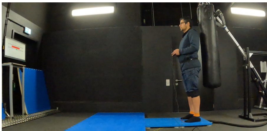
Figure 4. Experimental Setup. A participant is standing in front of the pushing machine, holding a joystick and engaging in a visuomotor task while waiting for the perturbation.
