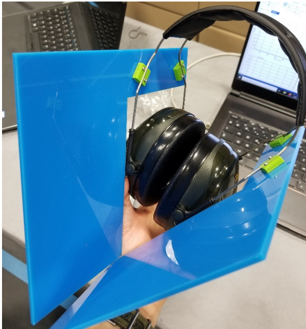
Figure 10. Picture of the sensory impairment device used during the experiments in order to change the level of awareness of participants regarding upcoming perturbations. The device was composed of a noise canceling headset with mounted plastic sheet on the side
