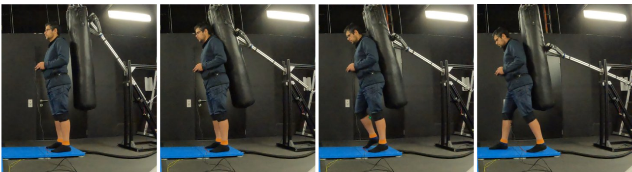
Figure 5. A sequence of one trial - waiting for a push while engaged in a visuomotor task, start of the push, start of the step, end of push and step.
